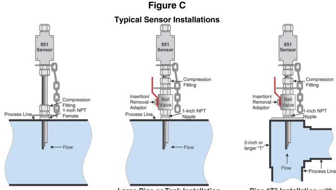
Large Pipe or Tank Installation
